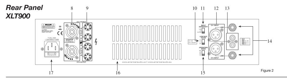
**8.** Channels 1 & 2 Speakon Outputs - Optional speaker output connections. Use pins 1+ and 1- of this 4-pole Speakon connector to connect to your speaker's Speakon input jack.
